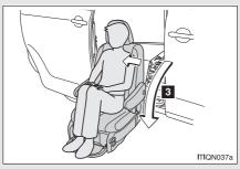
3 The AUTO ACCESS SEAT will slide out of the vehicle and will lower while the seatback raises.
