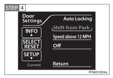
Choose a desired setting by pressing the "INFO" or "SETUP" button, then press the "SELECT RESET" button to select.
