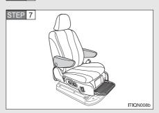
Adjust the armrest and foot restraint on the AUTO ACCESS SEAT to the downmost position.
