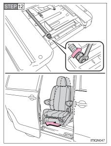
Turn the bolt with yellow marking clockwise using the combination wrench, and slide the seat until the marks are aligned as shown in the illustration.
