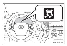
If the vehicle is in danger of slipping or if any of the drive wheels spins, the slip indicator light flashes to indicate that the Enhanced VSC/TRAC systems are operating.
