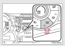
Turns the rear window and outside rear view mirror defoggers and windshield de-icer on/off.
