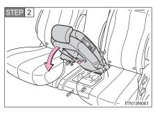
Unfold the cushion leg and push down on the seat to engage the front lock.
