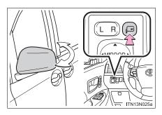
Press the switch to fold the mirrors.
