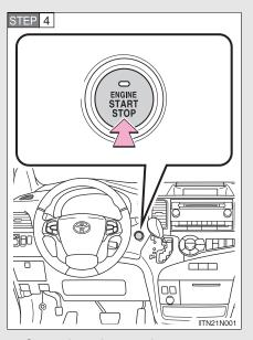
Press the "ENGINE START STOP" switch.
