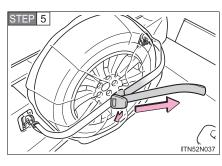
Pull strap to tighten and secure tire.
