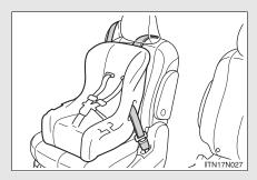
Seat belts equipped with a child restraint locking mechanism (ALR/ELR belts except driver's seat belt) (→P. 126)
