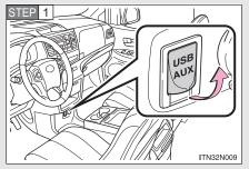
Open the cover and connect an iPod<sup>®</sup> using an iPod<sup>®</sup> cable.
