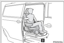
2 The AUTO ACCESS SEAT will rotate while the seat-back raises and while moving towards the rear of the vehicle.
