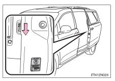
The sliding door cannot be opened by the inside door handle and the second seat sliding door switch when the lock is set.
