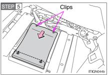
Remove the clips from the unit, and roll back the cover. ( $\rightarrow$ P. 57)
