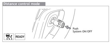
The distance control mode will cruise at a set speed, decelerate to maintain a selected distance from a slower vehicle traveling in front of you, and accelerate back up to the selected speed if the vehicle in front changes lanes or speeds up.
