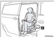
The AUTO ACCESS SEAT will rotate while the seat-back reclines and while moving towards the front of the vehicle.
