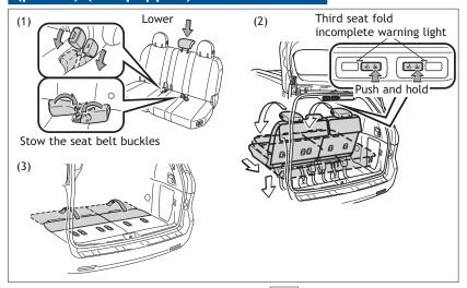
An alarm will sound for 10 seconds and the SEAT indicator will light up on the instrument panel if the seat is not fully open or stowed when vehicle is shifted out of Park.
