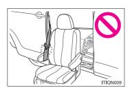
Before operating the AUTO ACCESS SEAT, make sure that the seat belt is unbuckled and that the seat belt is not tangled up with the seat.
