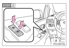
Shift the shift lever to P or N, and press and hold the door lock switch ( or or or approximately 5 seconds and then release.
