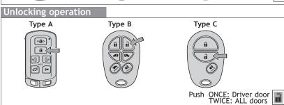
**NOTE:** If a door is not opened within 60 seconds of unlocking, all doors will relock for safety.
