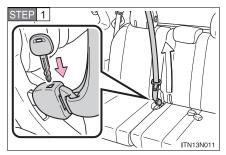
Insert the key into the hole on the center seat belt buckle to release the tab (with the hooked end), and allow the belt to retract.
