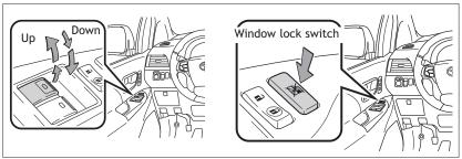
**Automatic operation** Push the switch completely down or pull it completely up and release to fully open or close. To stop window midway, lightly push the switch in the opposite direction.
