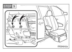
Use the combination wrench to remove the 2 bolts on the underside of the AUTO ACCESS SEAT.
