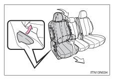
Pull the seatback angle adjustment lever and fold down the seatback. The cushion will tip up. The seat can slide forward.
