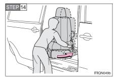
Rotate the seat into a position which does not cause the left edge of the seat cushion to make contact with the vehicle body.
