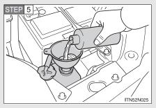
Add engine coolant if necessary.
