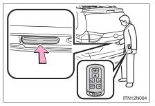
Press the unlock button to unlock all the doors.
