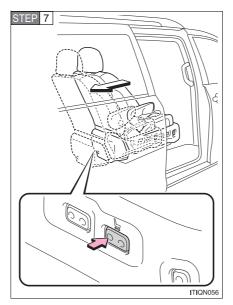
Press the rear side of the seat position adjustment switch on the right-hand side of the seat, and slide the AUTO ACCESS SEAT toward the rear of the vehicle until the beep sounds.
