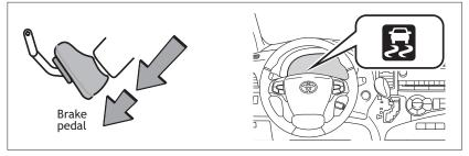
HAC helps prevent rolling backwards on an incline. To engage, push further down on brake pedal while at a complete stop until a beep sounds and slip indicator illuminates. HAC holds for approximately 2 seconds after releasing brake pedal.
