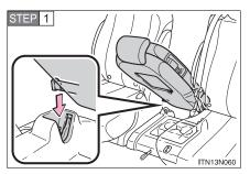
Engage the rear pins with the hooks.
