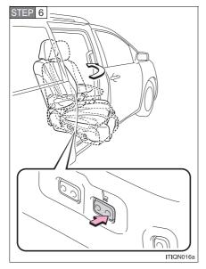
Press the forward side of the seat position adjustment switch on the right-hand side of the seat, and rotate the AUTO ACCESS SEAT toward the inside of the vehicle until the beep sounds.
