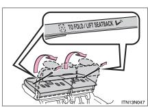
Pull the "TO FOLD/LIFT SEAT-BACK" strap, and raise the seat-back and the outside head restraints.
