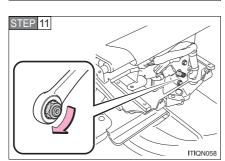
Turn the bolt with yellow marking using the combination wrench, and move the AUTO ACCESS SEAT until the bolt can no longer be turned.
