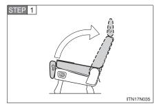
Fold down the seatback by pressing the folding/returning switch ( $\rightarrow$ P.104). Raise the seatback by pressing the same switch, the returning switch ( $\rightarrow$ P.108) or the seatback angle adjustment switch ( $\rightarrow$ P.95). (The seatback will automatically stop.) Do not touch the switch while the seatback is moving, because the operation will stop.
