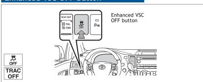
The Enhanced VSC OFF button is used to switch between modes related to the TRAC and Enhanced VSC functions.
