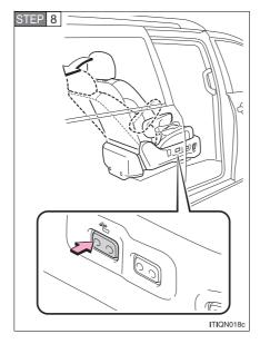
Press and hold the rear side of the seatback angle adjustment switch on the right-hand side of the seat until the seatback automatically stops moving.
