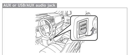
By inserting a mini plug into the AUX or USB/AUX audio jack, you can listen to music from a portable audio device through the vehicle's speaker system while in AUX or USB/AUX mode.
