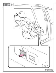
Press and hold the front side of the seatback angle adjustment switch on the right-hand side of the seat until a long beep sounds.
