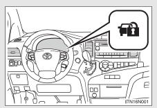
Close the doors and hood, and lock all doors. The system will be set automatically after 30 seconds.
