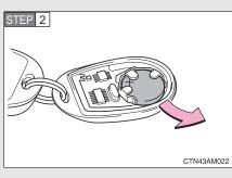
Remove the discharged transmitter battery.
