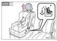
Secure the child restraint system using the seat belt or LATCH anchors, and adjust the head restraint to the uppermost position.
