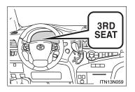
The warning light comes on if the third seat operation is not yet complete when the "ENGINE START STOP" switch is in IGNITION ON mode.
