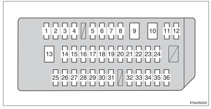
Fuse Circuit Ampere 1 P/OUTLET 15 A Power outlets Audio system, navigation system, 2 RAD NO.2 7.5 A rear seat entertainment system Main body ECU, clock, shift lock system, power rear view mirror 3 **ECU-ACC** 10 A control, multiplex communication system 4 CIG 15 A Power outlets Emergency flashers, buck up lights, navigation system, multi information display, automatic tran-5 **GAUGE NO.1** 10 A saxle, multiport fuel injection system/sequential multiport fuel injection system, charging system
