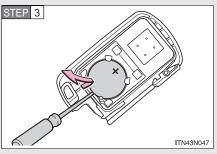
Remove the depleted battery.
