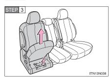
Pull the release lever under the cushion and simultaneously lift the seat to remove.
