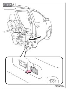
Press the rear side of the seat position adjustment switch on the right-hand side of the seat, and slide the AUTO ACCESS SEAT toward the rear of the vehicle by 2 in. (5 cm).
