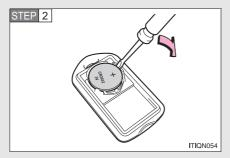
Remove the depleted battery using a flathead screwdriver.
