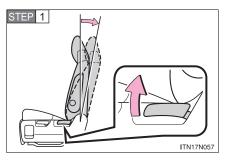
Fold the seatback while pulling the lever and move to the rearmost recline position.
