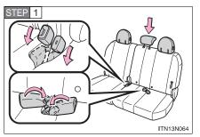
Lower the center head restraint to the lowest position, and stow the seat belt buckles.
