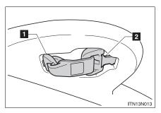
Pull tab 1 out and pull the belt out a little. Then pull tab 2 out.
