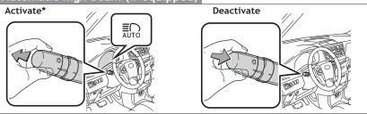
\* Refer to the *Owner's Manual* for details on activating the automatic high beams.
