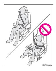
Wear the seat belt correctly, passing it underneath the armrest.
