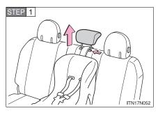
Secure the child restraint system using the seat belt or LATCH anchors. Adjust the head restraint to the uppermost position.
