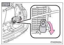
Remove the adapter socket.
