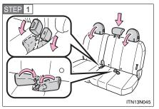
Fold the outside head restraints and lower the center head restraint to the lowest position, and stow the seat belt buckles.
