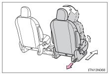
Pull the strap and fold down the seatback. The cushion will tip up. The seat can slide forward.
