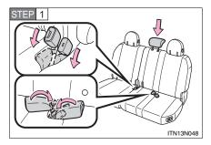
Lower the center head restraints to the lowest position and stow the seat belt buckles.
