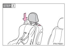
Adjust the head restraint to the downmost lock position.
