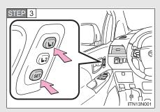
Press the "SET" button, then within 3 seconds press button "1" or "2" until the signal beeps.
