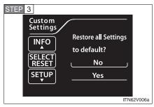
Select "Default Settings" by pressing the "INFO" or "SETUP" button, and press the "SELECT RESET" button.
