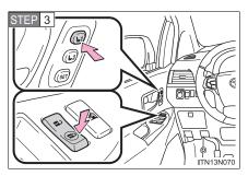
Press the desired button ("1" or "2") to recall the position. Then, while keep pressing the button, press the driver's door lock switches (either lock or unlock) until the signal beeps.
