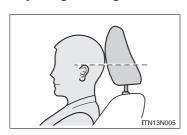
Make sure that the head restraint is adjusted so that the center of the head restraint is closest to the top of your ears.
