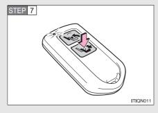
Press and hold the seat lower switch on the wireless remote control to rotate and lower the AUTO ACCESS SEAT.
