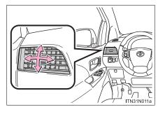
Adjusting: Direct air flow to the left or right, up or down.
