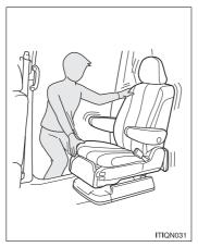
1 Shake the AUTO ACCESS SEAT gently to check that the seat is stowed properly. If not stowed properly, the seat may move unexpectedly, and could cause injuries.
