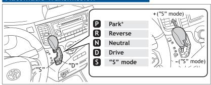
\* The "ENGINE START STOP" switch/engine switch must be "ON" and the brake pedal depressed to shift from Park.
