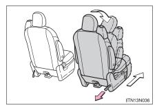
Pull the strap and fold down the seatback. The seat can slide forward.
