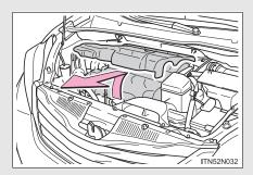
Lift the edge of the cover to fixed pins, and then pull the cover towards you to remove.
