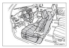
Exiting the vehicle: When all of the following actions have been performed, the seat will move backward (auto away function):
