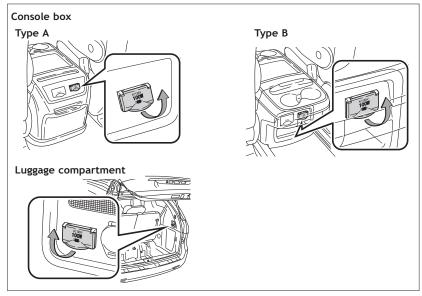
Designed for car accessories. Engine switch/"ENGINE START STOP" switch must be in the "ACC" or "ON" position to be used.
