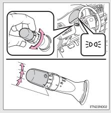
The side marker, parking, tail, license plate, daytime running lights (if equipped) and instrument panel lights turn on.
