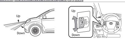
Rotating the dial downward will lower the angle of the beam.
