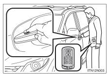
Touch the lock sensor (the indentation on the upper part of the door handle) to lock all the doors.
