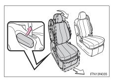
Pull the seatback angle adjustment lever and fold down the seatback. The seat can slide forward
