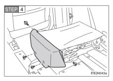
Remove the 4 clips and remove the unit cover. ( $\rightarrow$ P. 57)
