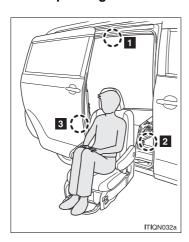
When operating the AUTO ACCESS SEAT, make sure that the occupant's head, arms and legs do not hit the door opening.
