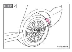
Slightly loosen the wheel nuts (one turn).
