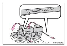
Pull the "TO FOLD/LIFT SEAT-BACK" strap and fold down the seatback.
