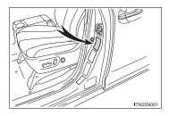
For the GAWR, see the Certification Label. For the maximum load of the tire, see the load limit at maximum cold tire inflation pressure mentioned on the sidewall of the tire.  $(\rightarrow P. 749)$
