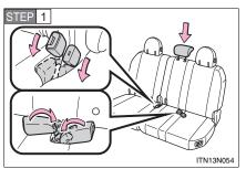
Lower the center head restraints to the lowest position and stow the seat belt buckles.
