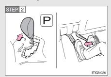
Shift the shift lever to P and set the parking brake.
