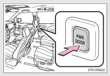
Press the switch to open and close each sliding door.
