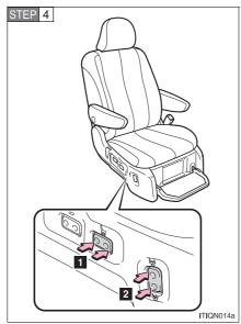
Press and hold the seat position adjustment switch on the right-hand side of the seat in either the front or back direction and, at the same time as press and hold the seat raise/lower switch in either the raise or lower direction for approximately 10 seconds, until the beep sounds.
