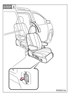
Press and hold the raise side of the seat raise/lower switch while the AUTO ACCESS SEAT raises, a short beep sounds, the seat slides further into the vehicle and a short beep sounds again.
