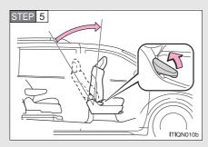
Fold the front passenger seatback while pulling the seatback angle lever.
